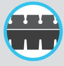
Anti-shear, dual hinge base allows greater contouring when the bed articulates, improving comfort and reducing shear forces.
